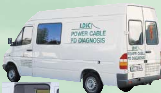
CDA-50 – Test Van for Power Cable Testing
