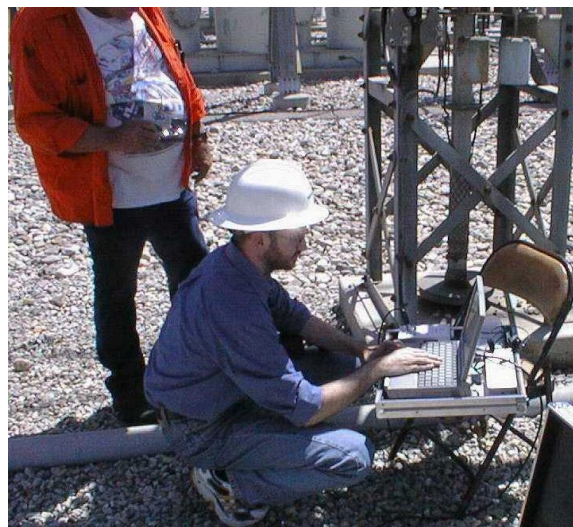
Figure 18: Digital On-Site PD Measurement
