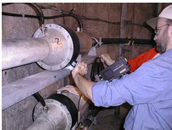
Figure 12: Cable Joint testing with the UHF-Sensor in a Manhole
