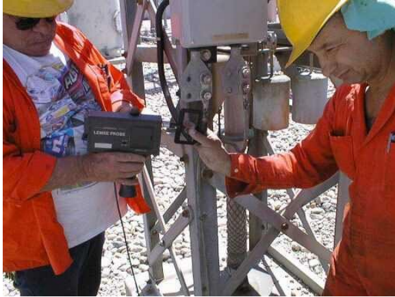
Figure 8: PD Measurement in a Substation
