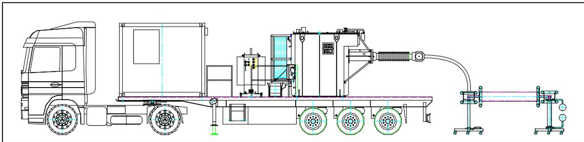
Fig. 2: Frequency-tuned resonant test system 90 A, 150 kV on a trailer with HV filter for PD measurement
