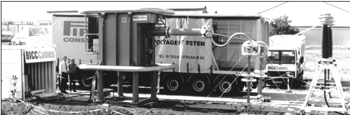
Fig. 3: Parallel connection of two identical test system 90A, 150kV to extend the available test current to 180A (By courtesy of BICC Cables Ltd., U.K. and Pirelli Construction Company Ltd., U.K.)
