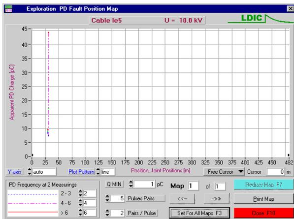
**Figure 5: PD fault position map**
