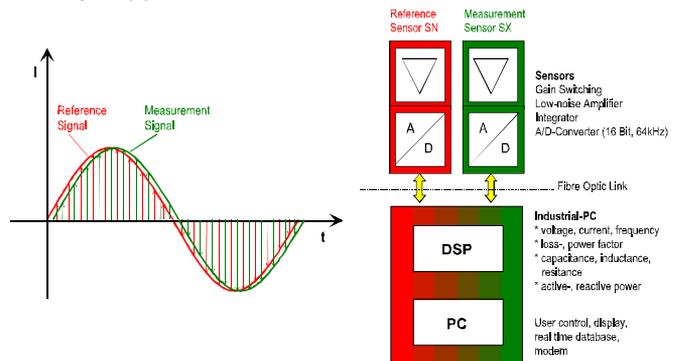
Figure 1: Concept of the loss / impedance measuring system
