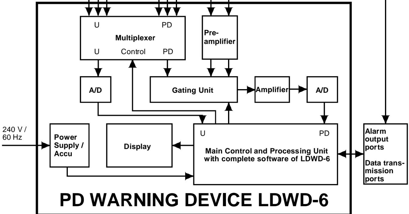
**Block diagram of the PD monitoring system**
