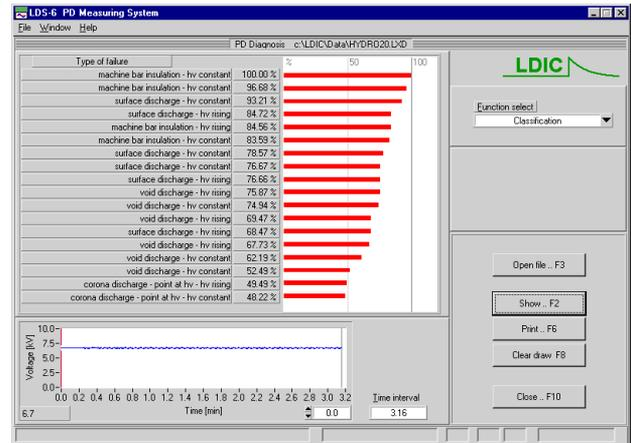
Figure 4: PD fault identification
