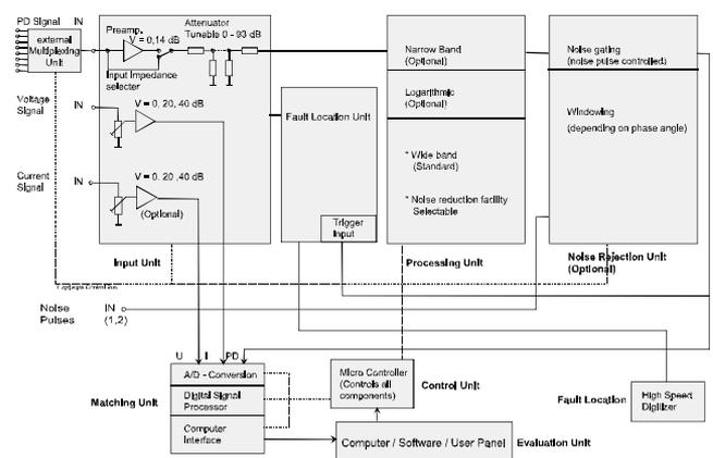
**Figure 3:** Schematic diagram of the PD-measuring unit
