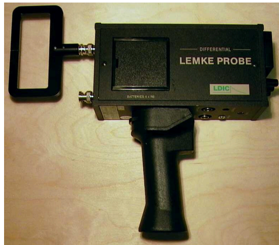
Figure 6: Lemke Probe LDP-5 with L-Sensor
