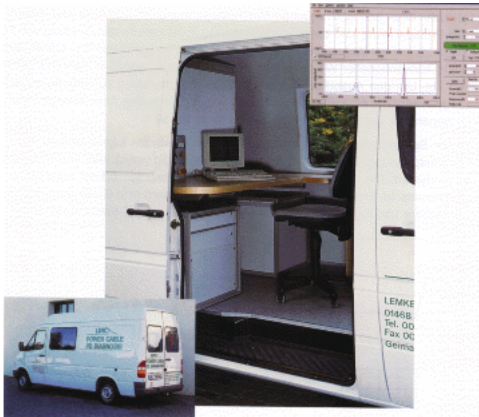
Fig. 1: View of the measuring and control modul of the CDA test facility, installed in a cable test van
